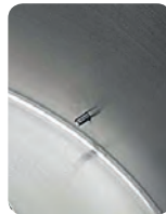
Second temperature probe directly in contact with the food.
