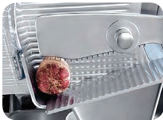
1. Fixing arm designed also for small sausages
