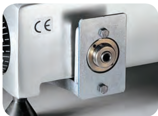
Device for releasing the carriage
