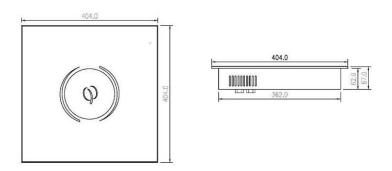
2. Dimension of the switch and small LED control box
