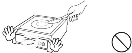
**WARNING : If the ceramic surface is cracked, switch off the appliance and unplug the unit to avoid possibility of electric shock.**
