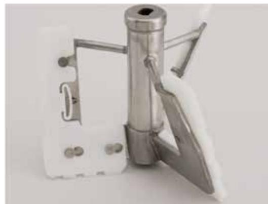
Removable and flexible agitator blade touches the vertical cylinder of the batch freezer to obtain a perfect mix during the working process.
