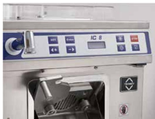
Digital microcomputer is easy to operate. Two set languages with the possibility to set the machine by timing or by degree to have a precise control of final product.
