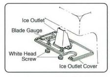
Loosen and remove the 2 white headed mounting screws by hand and remove ice outlet cover from body of unit.
