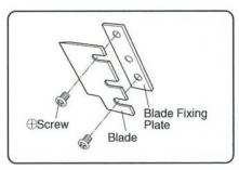
Loosen and remove the remaining 2 mounting screws between blade and blade fixing plate with a phillips **#**screw driver, and remove blade.
