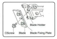
Fix a blade assembly into a blade holder with screwing 1 pce.(in the center) of its mounting screw.
