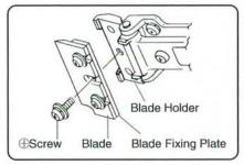
Of the 3 mounting screws between blade holder and blade, loosen and remove the middle screw (in the center) with a phillips ⊕screw driver, and remove blade and blade fixing plate.
