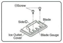
Push an blade to get a blade edge connected tightly/firmly against the side of © of blade gauge, and screw 2 pcs. (both ends) of their mounting screw(+) to re-assemble.
