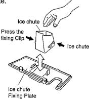
\* Clean Ice Chute with soft cloth or sponge. Shaved ice can be clogged if the inside surface of Ice Chute is scratched.
