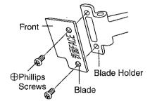
2) Fix Ice Chute Fixing Plate in reverse procedure of "Removing Blade".
